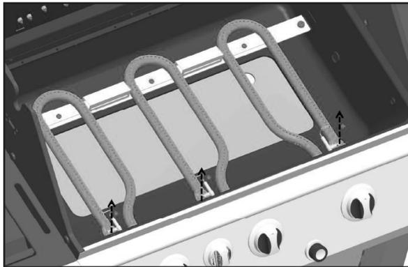
Remove the self tapping screw from each electrode as shown in **figure 2**.
