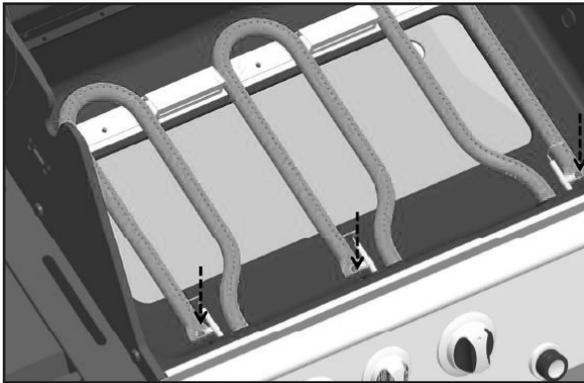
Place the new double burners into the burner box. Ensure that the venturi is seated correctly over the valve **figure 4**.
