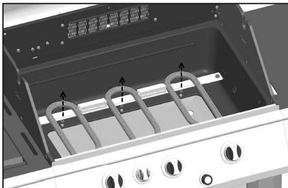
Remove the hardware used to attach the double burner to the carryover bar as shown in **figure 3**.
