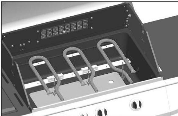
Use the new self-tapping screws to secure the electrode to the new double burner as shown in **figure 5**.
