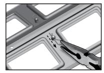
3. Remove the damaged Ceramic Stone and replace it.
